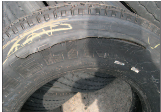
Fatigue Rupture or “Zipper”
